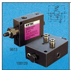
Sequence valves control the order of events within a hydraulic system by directing pressure to the two circuits in a pressure-controlled sequence. For example, this allows clamps to be actuated before work supports are locked.
