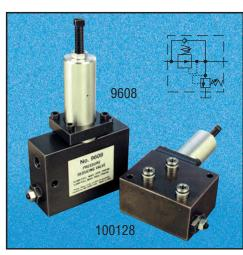
Pressure reducing valves are designed to reduce the maximum pressure in a portion of a hydraulic circuit: the valve is open from the inlet to the outlet until a pre-selected pressure is reached, at which point the valve closes to limit pressure in the secondary circuit. The need for a separate power source for each pressure level is eliminated.
