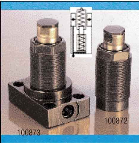
Hytec's fluid advance work supports have a spring loaded plunger which hydraulically extends to contact the workpiece. To support any externally applied loads, the sleeve surrounding the plunger grips the plunger and holds it in place.
