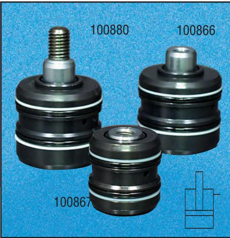
These "Pull" cylinders retract when hydraulically pressurized. They were created to permit the user to design a cylinder into a fixture while maintaining the replaceability and long life of a heat treated, corrosion resistant cylinder body. Typical applications of these cylinders include installation behind fixture plates or buried in tombstones where they can supply clamping force without taking up valuable fixture space.
