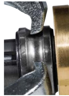
Lock on ball grooves and bearing races.
