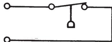
**NOTE:** Switch is wired normally open and held closed by spring force.
