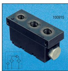
Hytec's pilot operated check valve offers a unique poppet seal design making them ideal for pallet applications or other specialized control circuits where zero leakage is essential. They can be used in any application where pressure must be maintained in a portion of a circuit until a separate pilot signal opens the valve and allows free flow in the reverse direction.
