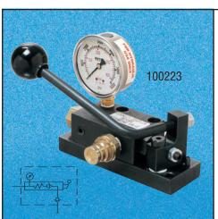
This valve allows the hydraulic power source to be disconnected after the fixture has been clamped. As the system is pressurized, the valve automatically closes to maintain pressure without manual intervention, and a liquid filled gauge lets you constantly check system pressure.
