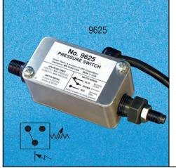
This hydraulic pressure switch is used to either control or monitor system pressure. To control system pressure the switch can be electrically wired into a pump's power circuit. At lower pressures, the switch is closed, causing the pump to run. When the pressure reaches the switch setting, the switch contacts open, stopping the pump. When system demands cause the pressure to drop 300 psi, the contacts will again close to start the pump. This switch is included with all Hytec electric pumps.
