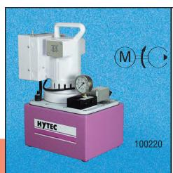
This electric/hydraulic pump is a two-stage, continuous pressure (demand) pump that contains all the necessary controls and circuitry for powering any single- or double-acting continuous pressure workholding system. It has a pressure switch and an external pressure regulator, both infinitely adjustable throughout the operating pressure range of 1,000 to 5,000 psi. An internal safety relief valve prevents damage from exceeding the maximum rated pressure.
