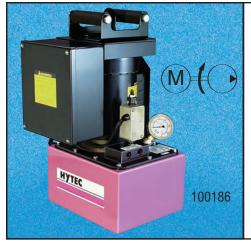
These electric/hydraulic pumps are twostage, continuous pressure (demand) pumps that contain all the necessary controls and circuitry for powering any single- or doubleacting continuous pressure workholding system. They have a pressure switch and an external pressure regulator, both infinitely adjustable throughout the operating pressure range of 1,000 to 5,000 psi. An internal safety relief valve prevents damage from exceeding the maximum rated pressure.
