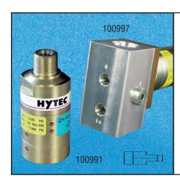
Intensifiers are used in applications where an existing low pressure hydraulic source is available. They amplify low pressure to a range better suited to workholding systems
