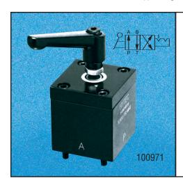
Similar to Hytec's 100969 and 100970, this 3-way/4-way, two-position directional control valve is ideal for manifold mounting on your fixture. The valve's zero-leakage design is the right choice for constant pressure applications. Its smaller size allows you to maximize usable fixture space.
