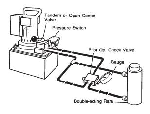
Double-acting cyinder with remote control valve and a remote pilot operated check valve. (Holds cylinder pressure when valve lever is in neutral postion.)
