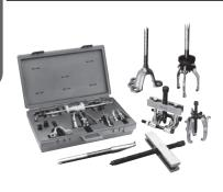
Components can be assembled to create several versatile puller versions. The puller head is turned to securely lock the jaws onto the part being removed. Both a 2-way and 3-way puller head are included, plus three long-reach and three short-reach puller jaws in a plastic storage box. Easily removes gears, bearings and other press-fitted parts.
