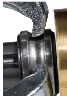
Lock on ball grooves and bearing races.
