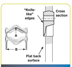
Attachment clamps down into V-groove to distribute load. Use with Lock-Jaw™ pullers or Bi-Directional™ Pullers.
