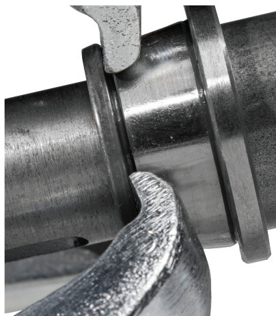
Tapered roller bearing on shaft.
